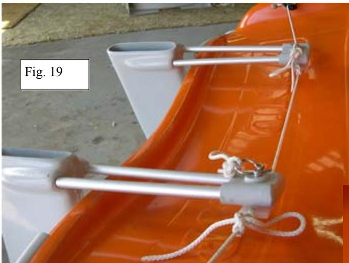
6.3 Remove the spring clips and pass the clevis pins up through the holes at the end of the tillers. Re-insert the spring clips. (fig 19)
